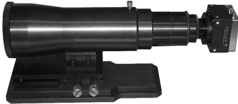
Fig. 4. Photography of our Shack-Hartmann wavefront sensor
