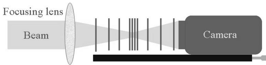
Fig. 1. Principle of  $M^2$  measurements
